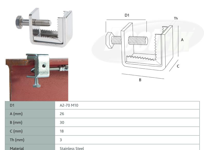
Used as corner fixings for perimeter wire rope netting frameworks
